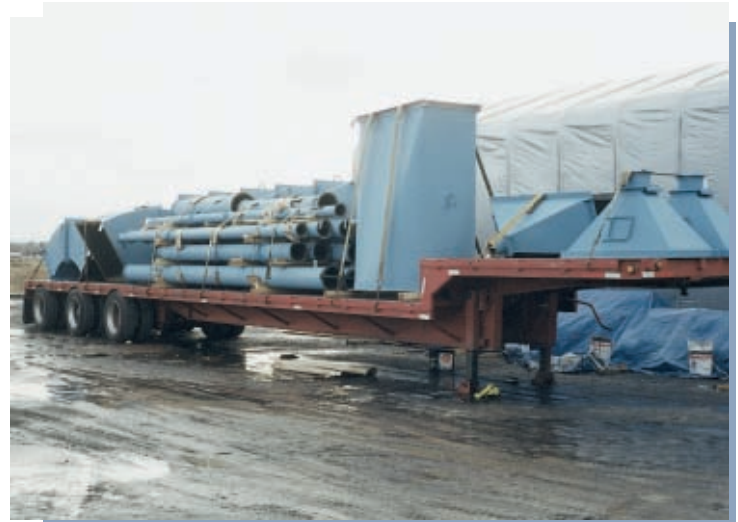
Ducting including Stacks, Diverters, Dampers, Hoods, Cyclones, etc.
